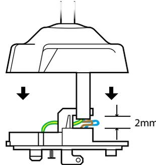
4. Terminate conductors into terminals.
